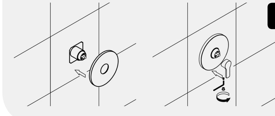
Use the screws to fix on the wall the built-in mixer box.
