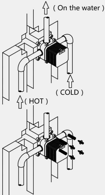
After the pipe connection, according to the pipe arrangement, make a slot in the wall for the connection.
