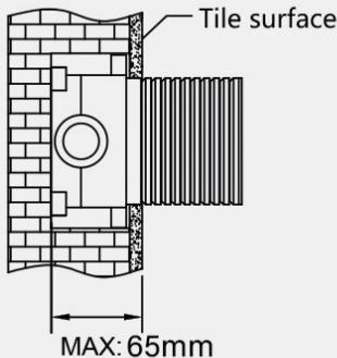
Pay attention for a correct installation of the built-in mixer box. Hot water inlet is on the left.
