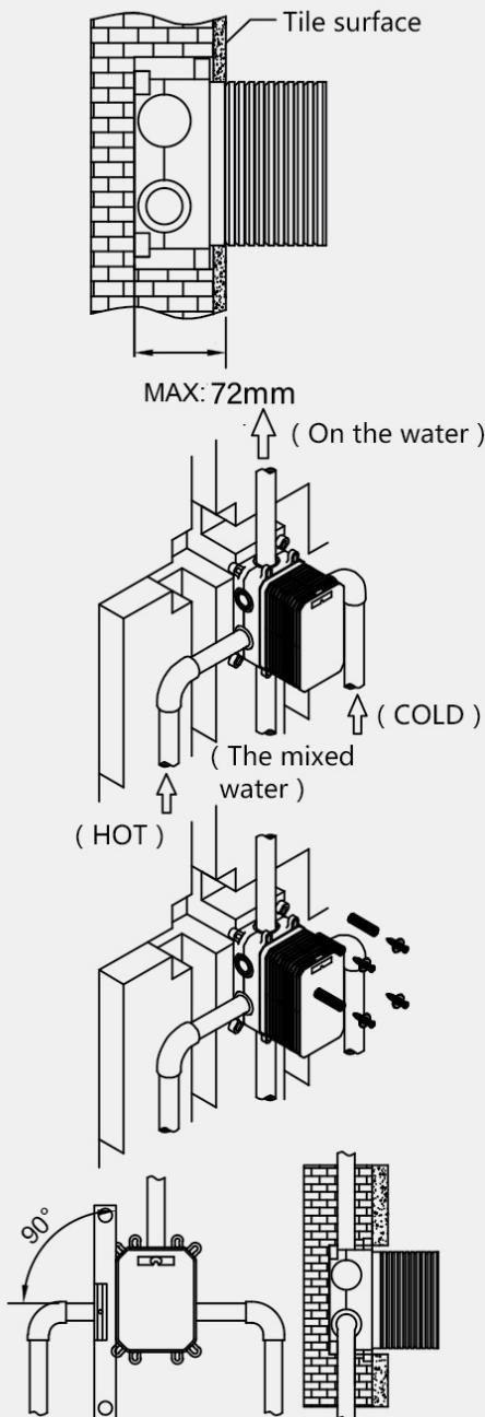
Pay attention for a correct installation of the built-in mixer box. Hot water inlet is on the left.
