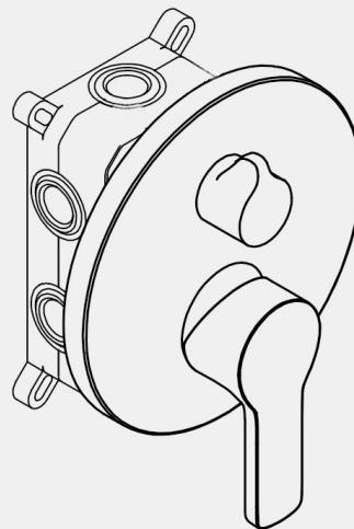
The bottom of the hole should be flat for a correct installation of the built-in mixer box. Recommended sizes: 160 x 100 x 65 MM.
