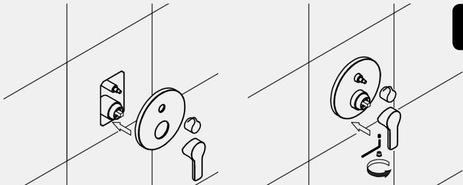
Use the screws to fix on the wall the built-in mixer box.
